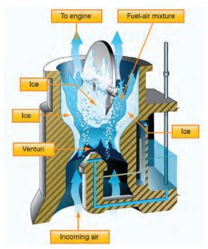
The formation of carburetor ice may reduce or block fuel/air flow to the engine.
