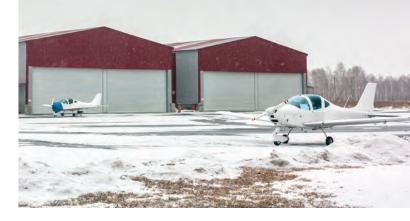
To find out what else goes into successful aircraft winter storage, I talked to Gary Suozzi, aviation safety inspector with the FAA's Aircraft Maintenance Division. Suozzi outlined some basic steps to remember like chocking the wheels (front and back) and making sure to release the parking brake.
