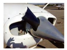
To avoid damage like this Cessna 172 prop, always check carefully for cracks
