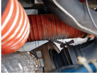
Evidence of an exhaust leak can be seen on nearby components.
