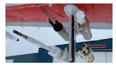
Instruments attached to the wing — including (counterclockwise from upper left) a forward scattering spectrometer probe, Rosemount air data probe, and cloud droplet probes — measure different cloud particle sizes and concentrations.
